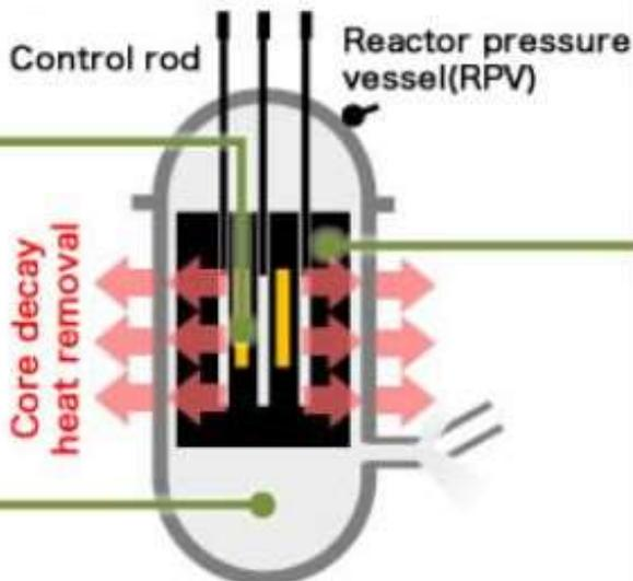
Radionuclides can be retained within the plant by inherent reactor shutdown and core cooling without any equipment or operator action in case of loss of coolant accident or station blackout.
