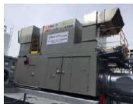
Hydrogen Gas Turbine (1MW class)
